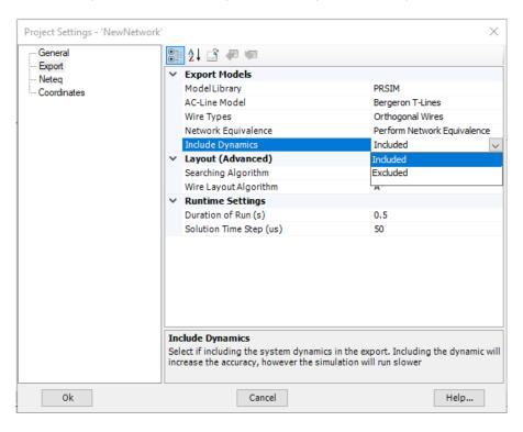
Applying system dynamics will replace a network element such as ideal AC source with its equivalent dynamic model which may be a combination of a synchronous machine, exciter, turbine, and governor as shown below.
